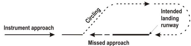
**Note:** the indicated situation is applicable for an initial instrument approach to RWY 06. Circling approaches southeast of RWY 06/24 and extended centre line are prohibited.
