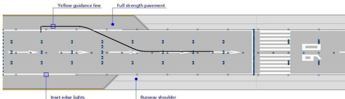
No turn-around area is provided at the end of RWY 18L. Marshaller guidance is required for aircraft with wingspan 36 M or greater and available on pilot's request. A tow truck is required for EASA code letter F aircraft, or at ATC discretion.
